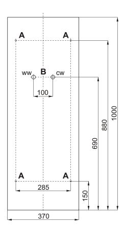
A - holes with diameter 8 mm for strut studs
